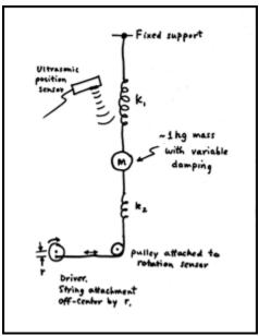
A steel mass is suspended from a fixed support with a spring  $(k_1)$ . A driver is attached from below using a weaker spring  $(k_2)$ . With this setup you have a very stable driving amplitude and frequency, the ability to observe large changes in oscillator amplitude, and a damping constant that can be controlled over a range greater than 1000.
