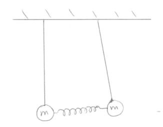
Double pendulums folded up and held together with a rubber band "double" as physical pendulums. Each physical pendulum is mounted on a Pasco Rotary Motion Sensor. Light ( $k \sim 3 \text{ N/m}$ ) springs couple the pendulums. The position of the spring along the length of the pendulum determines the strength of coupling.
