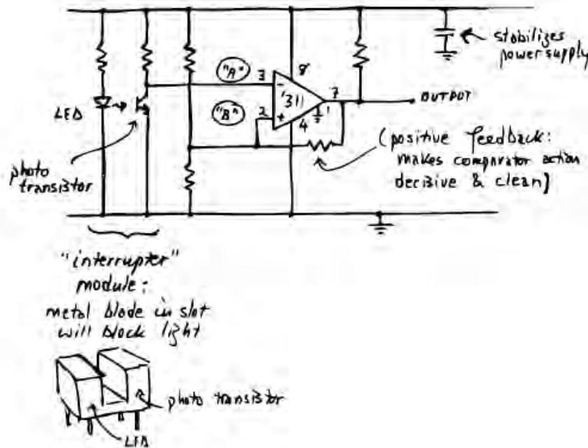
Figure 2: Timing circuit used in Lab 1
