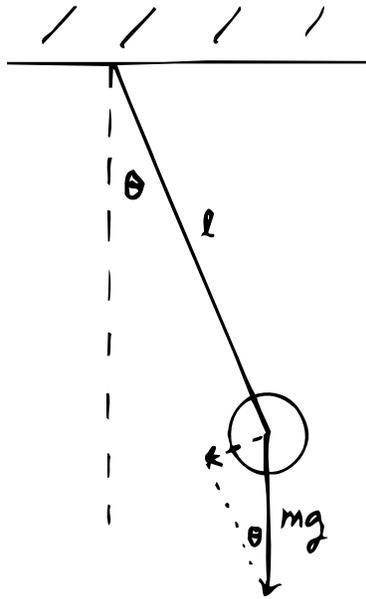
**Figure 1: Forces on a simple pendulum**
