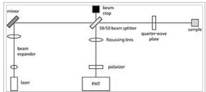
Figure 8. Coherent backscattering schematic.
