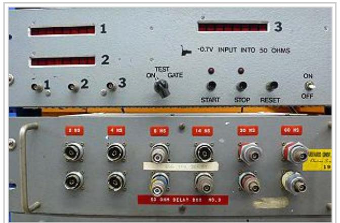
Figure 7. Homemade scaler and coaxial delay box
