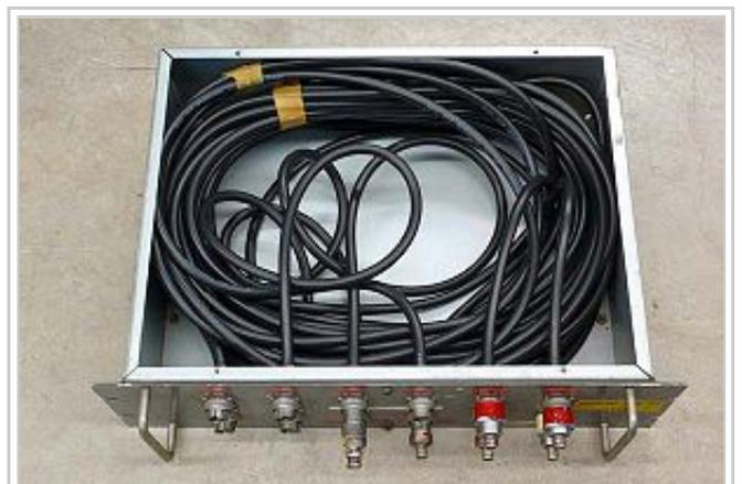
Figure 8. Coaxial delay box
