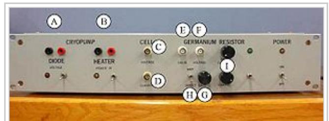
Figure 7. Heat capacity interface box panel
