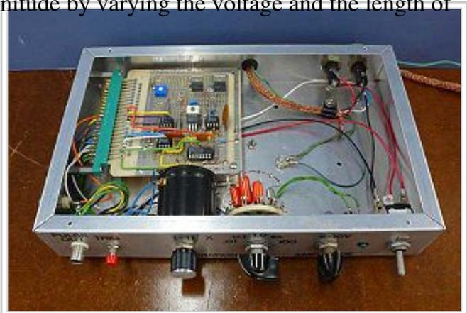
Figure 9. Heat capacity pulser - circuit view
