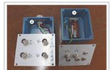
Figure 5. Second sound breakout box and DC current source
