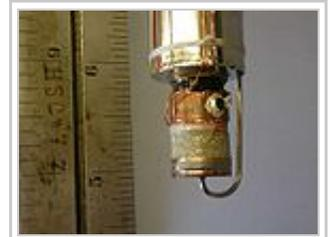
Detail of sample can showing capillary, heater and diode.
