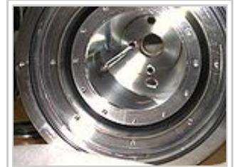
Bottom view of cryostat body with sample can removed.
