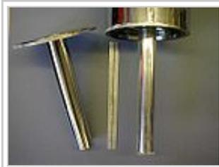
Aluminum radiation shield, bolted to nitrogen can. Tail cap has been removed.
