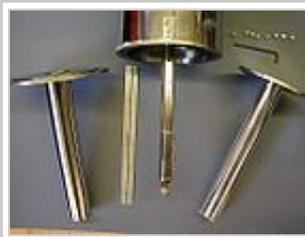
Sample can. Radiation shield has been removed.
