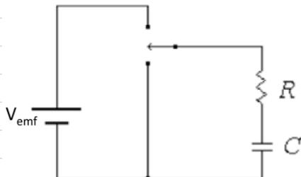
where:  $R = 30 \text{ k}\Omega$ ,  $C = 1 \text{ }\mu\text{F}$ , and the battery is a standard 1.5-volt AA cell battery.
