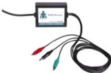
The EKG sensor plugs into one of the sockets on the left side of the LabPro. It has three alligator clips, colored red, black, and green.
