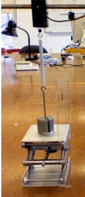
5. Measure the height of the lab jack above the table, and measure the spring force using the force sensor. The meter on the Logger Pro screen will probably jump around a little bit, but you can easily estimate it to the nearest 0.1 N.
