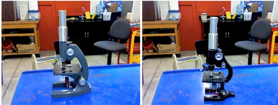
2. The microscopes have been fitted with an LED light source and a modified iSight camera. The microscope objective will cast an image of the sample on the slide directly onto the CCD array of the camera; illumination is provided from below the microscope stage by the LED. From this setup, Logger Pro can capture time-lapse video of Brownian motion of particles suspended in solution on the microscope slide.
