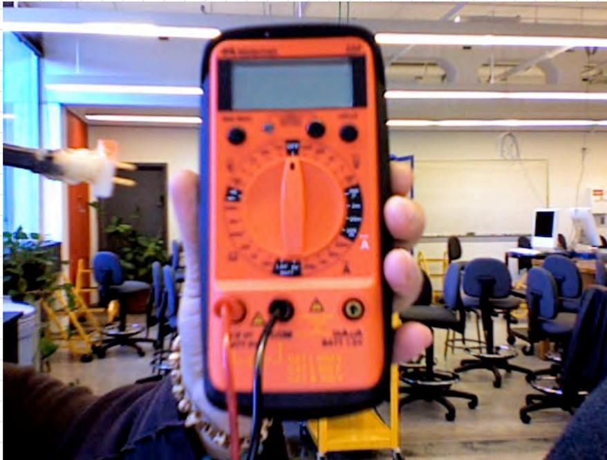
2. Depending on the model of multimeter, you may also have to set the range of the instrument. For the purposes of this lab, you should use the 20-volt setting.
