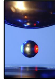
This is a close-up of a sample of titanium-zirconium-nickel alloy inside the Electrostatic Levitator (ESL) vacuum chamber at NASA's Marshall Space Flight Center (MSFC). The ESL uses static electricity to suspend an object (about 3-4 mm in diameter) inside a vacuum chamber allowing scientists to record a wide range of physical properties without the sample contacting the container or any instruments, conditions that would alter the readings.
