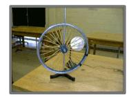
Shine a heat lamp onto the rubber bands on one side of the heat engine. As the rubber bands are heated, they contract, moving the center of mass away from the center of rotation. This causes the engine to rotate!
