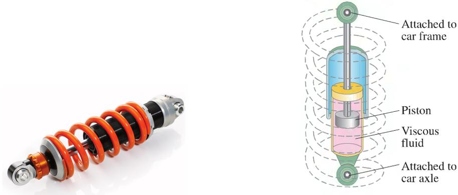
Figure 1: A picture and schematic of a spring and a shock absorber.
