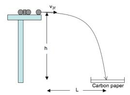
• The track is positioned so that it ends right at the edge of the lab bench. Ball 3 will be launched off the end of the track, and it will strike a piece of carbon paper on the floor, leaving a dark mark. If we measure the height of the bench h and the horizontal distance L from the end of the track to the mark on the paper, we can calculate the velocity with which the ball was launched (assuming it is initially moving in a purely horizontal direction).
