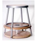
Use this four-legged stool that sits on a rotating platform with low friction to explore angular momentum phenomena, and to measure your moment of inertia.
