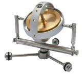
Use this gyroscope on a gimbal mount that allows it to rotate freely along two axes of rotation (horizontal and vertical) to explore the phenomenon of precession.
