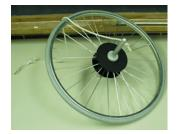
This bicycle wheel has handles along the axis of rotation so you can hold on to it while it spins. Use it with the spinning stool to explore (and experience!) conservation of angular momentum and precession.
