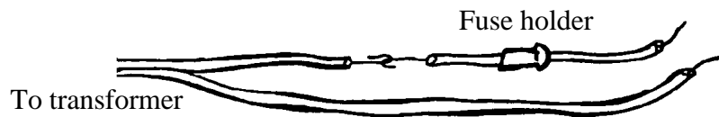
Figure 7: stripped wire and fuse holder
