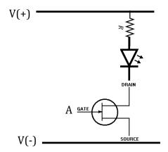
Build the following circuit using the FET (field effect transistor) and LED (light emitting diode) provided. The LED should have a 100 ohm resistor in series it to limit the current and preserve the transistor and LED. Find the IV curves for the drain to source when A is held to a low potential (ground) and then for A held to a high potential. Include your graphs here.
