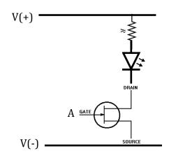
Build a transistor circuit on the breadboard. Place the drain at a high potential (5 V) with a 100 ohm resistor to limit the current. Place the source at the ground. The Gate (input = A) voltage will be switched between the high and the low potential. Watch the output of the circuit with the LED .
