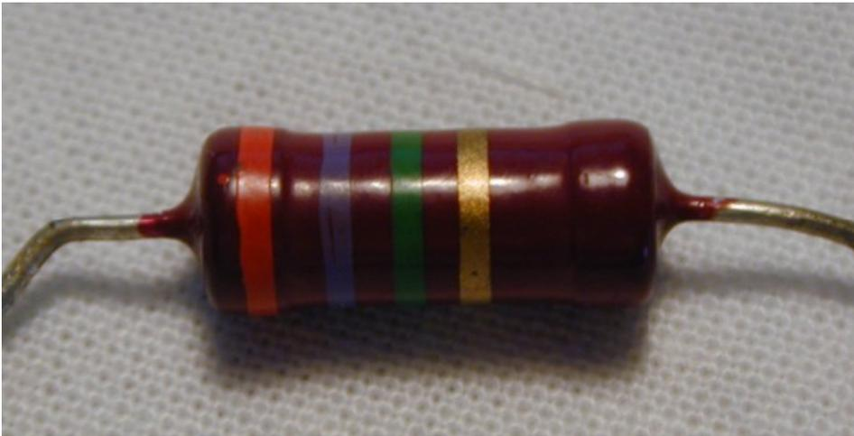
If you are not sure which end to start from, most resistors have a gold or silver band as their fourth band to indicate tolerance.
