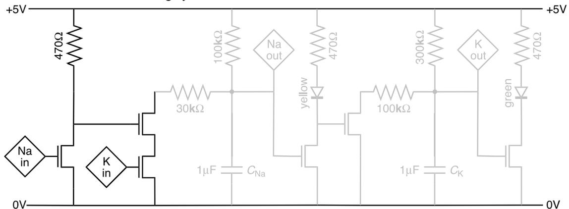
The point labeled "Na in" should have a long **yellow** wire sticking up out of the board, while the point labeled "K in" should have a long **green** wire sticking up out of the board.
