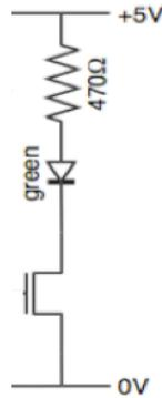
Take a long orange wire and connect one end to the gate of the transistor and the other end to the +5V rail. Plug in the power supply. The LED should be on—if it is not on then unplug the power supply and check your wiring (make sure the LED is oriented properly, with the long leg connected to the resistor).
