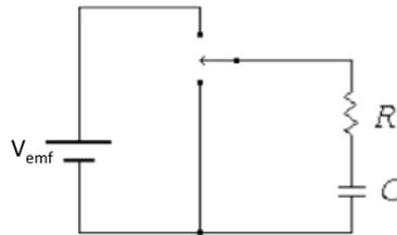
right, where:  $R = 30 \text{ k}\Omega$ ,  $C = 1$  AA cell battery.
