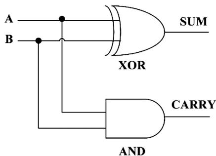
Build a half adder from what you already have on the breadboard and verify it works as expected. **Show your TF. Draw out a truth table for 4 columns (A, B, Sum, Carry) and fill it out, then take a picture and paste it below.**
