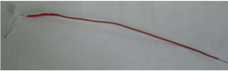
This is a device consisting of two LEDs (light-emitting diodes) in a single plastic dome on a long wire. It is used to probe the digital voltage in a circuit. The long leg should be plugged into the far right of your breadboard between two resistors. The other end (the leg of the LED itself) is the terminal you'll use to probe your circuit.
