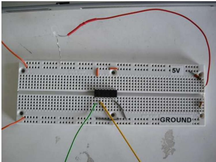
On a breadboard you'll be given an XOR gate which is actually made out of an integrated circuit, or IC (the black chip in the middle of the breadboard). It would require quite a few transistors to make an XOR yourself, but the chip actually contains four separate implementations of XOR inside it. You'll only need to use one. The leads connected to the two leftmost pins on the bottom row are the inputs; the next pin over (3rd one on the bottom) is the output.
