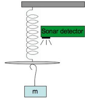
Remember, the sonar detector can only detect objects a *minimum distance of 15 cm away*. Also, use only small amplitudes of oscillation; this will significantly decrease the chances of having the mass fall off the stand and break something and it gives cleaner data.
