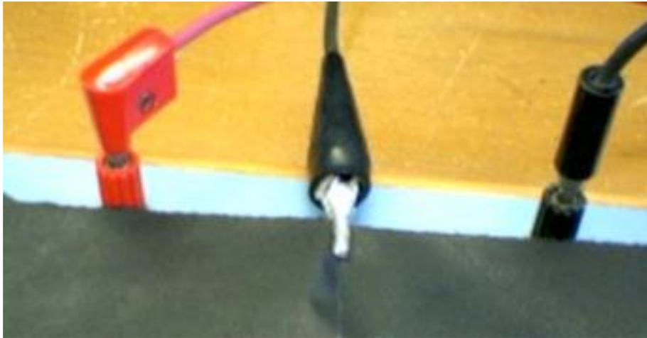
5. Using the red probe of the multimeter, measure the voltage of the positive and negative terminals of the board relative to the point halfway in between them where you clipped the alligator lead. Adjust the position of the alligator clip until you get approximately equal magnitude with opposite sign values for the voltage on the terminals.
