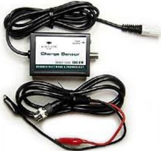
It acts almost exactly like the differential voltage probe, except that its "internal resistance" is much higher, so that it won't discharge a capacitor while you are trying to measure its voltage. The downside is that the charge sensor has an internal time constant of 0.1 s, so you can't use it to measure anything that changes more rapidly than that.
