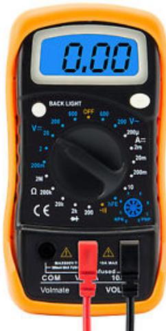
A multimeter is an important tool to measure electronic components and circuits. The ground or COM port (black) and high voltage (red) port have electrodes already connected for you. We will need to perform two types of measurements: Voltages (turn dial to "V") and ohmic resistances of resistors (turn dial to " $\Omega$ "). Make sure to start with a large range and decrease the range stepwise to get a better resolved value. A "1" on the display typically indicates that your range is too small.
