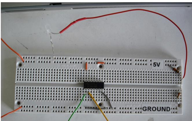
On a breadboard you'll be given an XOR gate which is actually made out of an integrated circuit, or IC (the black chip in the middle of the breadboard). It would require quite a few transistors to make an XOR yourself, but the chip actually contains four separate implementations of XOR inside it. You'll only need to use one. The leads connected to the two leftmost pins on the bottom row are the inputs; the next pin over (3rd one on the bottom) is the output.
