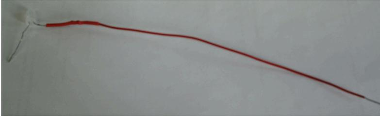
This is a device consisting of two LEDs (light-emitting diodes) in a single plastic dome on a long wire. It is used to probe the digital voltage in a circuit. The long leg should be plugged into the far right of your breadboard between two resistors. The other end (the leg of the LED itself) is the terminal you'll use to probe your circuit.
