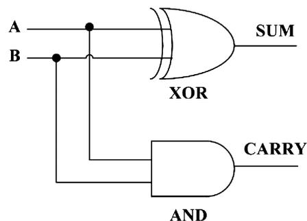
Build a half adder from what you already have on the breadboard and verify it works as expected. Show your TF. Draw out a truth table for 4 columns (A, B, Sum, Cary) and fill it out, then take a picture and paste it below.
