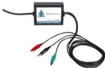
The EKG sensor plugs into one of the sockets on the left side of the Lab Pro. It has three alligator clips, colored red, black, and green.
